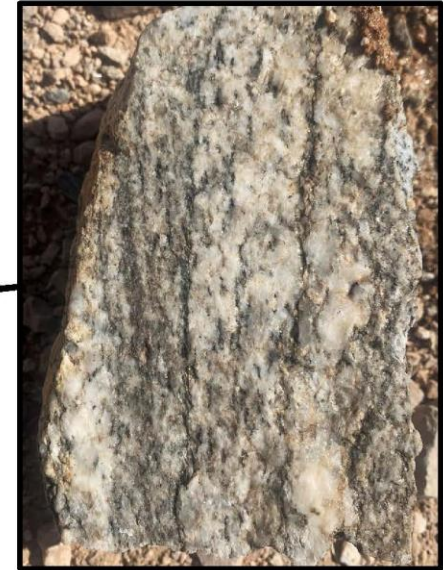
Iron oxide + kaolinite alteration in Bear Canyon conglomerate.
